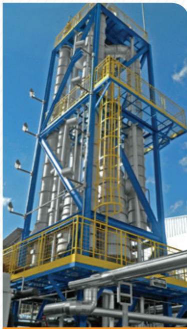
TASTE® Evaporator for orange juice installed in Cooperativa Integrada in the city of Uraí/PR - Brazil
