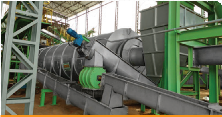
Citric bagasse dryer with multiple turns, installed at Citrus Juice, in Itajobi/SP - Brazil
